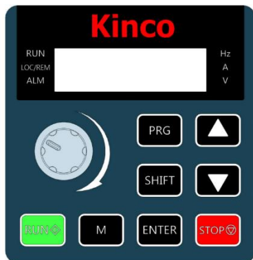
Figure 4-1 Schematic diagram of the LED operating panel
