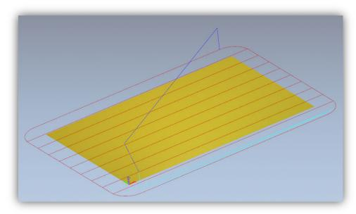
Now we record the trajectory, go to the Toolpaths tab and click the icon. In the record window, select so-called postprocessor, to define output data format suitable for our control system. In ArtCam we recommend "G-Code Arcs (mm) (\*.tap)". It is basic G-Code format suitable for Mach3 program. When you select the format pres "Save" and save our trajectory as e.g. "planning.tap".
