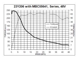
low – something about 200 rpm - the torque is almost the same (pictures below), but with increasing revs the torque, actually the power on the motor shaft), decreases drastically. It decreases to such low value that sometimes happens that at 1000 rpm. the motor has no power to work itself, not saying about propelling the machine.
