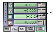
After this operation, we can start work from the second file not forgetting about the measurement after tool change ("Auto Tool Zero" button).
