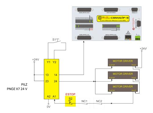
Above you can see an example of E-Stop signal connection to the CSMIO/IP-S controller and to the axis drives, using Pilz company safety relay (PNOZ X7 24V symbol). S1 is a reset button (switching on the safety relay), S2 is the emergency stop.
