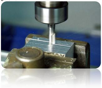
You can change the tool for an engraving cutter and load the second, previously generated trajectory. Before processing, there is one important detail. When planning the surface we lowered its level, the engraving logo would be 0.1mm depth, and not 0.3mm like the one we had assumed. "This can be easily remedied by reducing the zero point level about 0.2mm (planned depth). Click on the text box that displays current Z position and type on your keyboard "0.2 <enter>".
