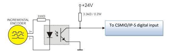
In this case, we must use directly the encoder signal or servo drive TTL encoder output. Aesthetic connection will be in this situation a little troublesome.
