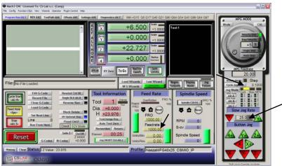
Now use arrow keys or keys on a machine desktop, reach left edge of the material. Z-axis is a little below the material level.
