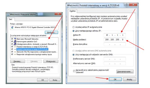
Double click on TCP/IPv4 protocol, and next enter the address IP: 10.1.1.1 and network mask: 255.255.25.0. Confirm with OK.
