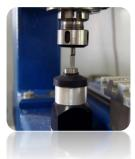
As it was mentioned at the beginning – to set the material base we are going to use the carbide roller, filed precisely on half of diameter. If we use tool length measurement, then enter the tool
