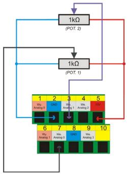
As you can see on the scheme - having 10V on an analog connector is very comfortable – thanks to it, we do not need any external power to supply potentiometers. Potentiometer 1 was connected to analog input no. 0, and potentiometer 2 to analog input no. 1. After connection you can check it by analog inputs preview in diagnostic window – menu "PlugIn Control —> CSMIO\_IP plugin", "Analog IO" tab.
