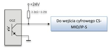
As it is shown - pull-up resistor is enough. However sometimes we do not have "open collector" – type output available, then the only way for homing on index is to add external, simply electronic system:
