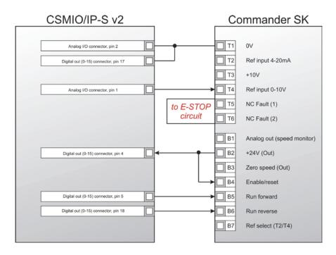
In the example above, you can see the simplest connection of an inverter to operate spindles in an engraving plotter.
