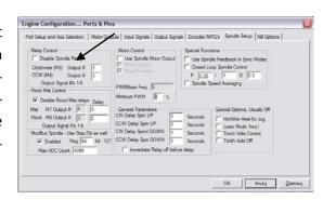
There are two options: for right revs (M3) and left revs (M4). We must uncheck "Disable Spindle Relays" box of course - that means no support for spindle activation.
