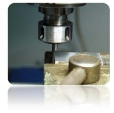
At this point, we can set the material base in X-axis by clicking "Zero X" button on the Mach screen. Coordinate X on the screen will be reset.
