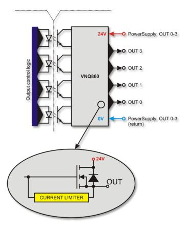
If we do not care about CSMIO/IP controller and digital outputs supply potentials separation and we want to use one supply source then we can link power supply of all the groups (pins 1, 4, 7, 10) and connect to controllers +24V supply. Of course you must also connect supply primary lines, 0V (pin 14, 17, 20, 23) to GND of CSMIO/IP controller power supply.
