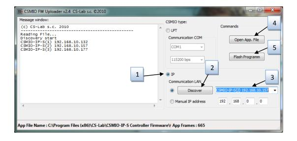
If you run the update application from installer file it means that correct file with the firmware was already loaded and "Open App. File" button is not active. If there is only one CSMIO/IP controller in network - the application asks to start the update automatically. If there are more controllers then you should chose one IP address from a list to update the controller you want and click "Flash Program".
