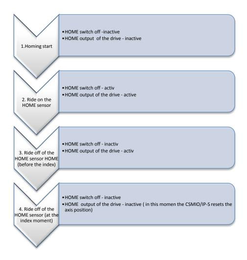
As shown on the diagram above, the drive should extend the active state on the HOME output until it step on the encoder index. During the tests with ARBAH drive the achieved homing accuracy at 2000mm/min speed and encoder's 10000imp/rev - ranged +/-1 imp. of the encoder.
