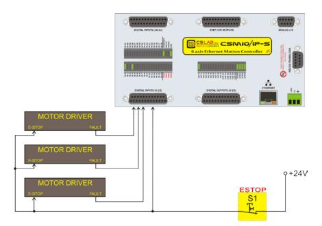
In the example above we used direct emergency signals connection. Such a connection is very easy and at the same time, it ensures satisfying safety level. Of course, the easiest way is to connect the E-Stop only to CSMIO/IP-S but then we lose double protection and it is no longer so safe solution.
