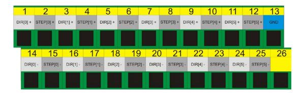
By default, axes are assigned to following channels STEP/DIR:  $X \rightarrow [0] / Y \rightarrow [1] / \text{etc.}$
