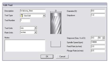
treatment last longer. Feed Rate is a feed on XY surface, and Plunge Rate means speed with which the tool will get into the material. Tool Type is a tool shape type. Here the drawing, displayed after shape type selection, is helpful.
