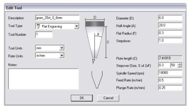
You should note that, in ArtCam program a handle size is given as diameter, and a dimension of tip of the tool (F) is as radius. Speed values in here are quite low but it is only example, and not "high performance ride",
