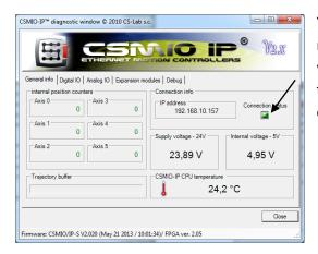
You will see CSMIO/IP diagnostic window. If the "Connection status" light is green it means that the software is installed correctly and communication between Mach3 program CSMIO/IP controller is also correct.
