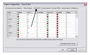
Configuration of the input signals we call from menu "Config—Ports and Pins", by selecting "Input Signals" tab. A list of standard input signals will appear and you can assign these signals to hardware inputs of CSMIO/IP-S controller.
