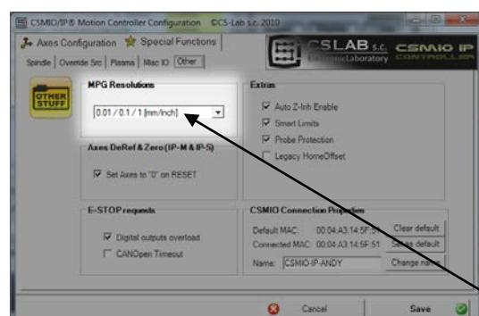
You can select it in the plugin's configuration - “Config/Config Plugins” menu, click “CONFIG” area, next to the CSMIO-IP-P-CS-Lab-s.c.” and go to "Other" tab. In the “MPG Resolutions” group select the desired multipliers
