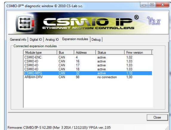
Next – in the Mach3 program- turn on the MPG function. To do this – click on the “Config/Ports and Pins” and go to the “Encoder MPG’s” tab and select MPG#1.
